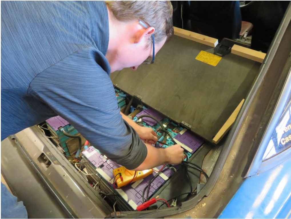
A student checks the voltage output on a battery pack in the electric car.
